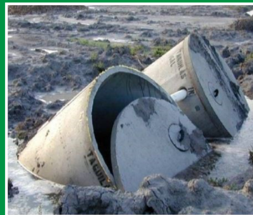
Empty tanks can become buoyant during flooding and cause serious damage.
